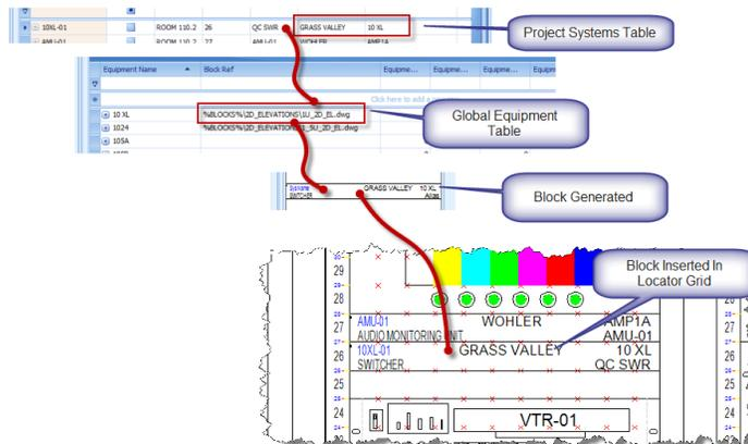
Assuming all of the data fiddly-bits are in the right place, the Rack Builder tool will populate the drawing with one locator grid per location selected. A locator grid is an array of point entities that are spaced horizontally and vertically based upon your selection in the preferences.
