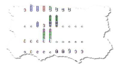
After running the RatsNest tool. This supplies the drawing with cable data and provides a positional reference to help you decide where to move block to better display the drawing.
