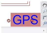
2. Select the **Arc Distance** and **Self-Connect Arc Dist.** **Arc Distance** sets the polyline bulge factor. An Arc Distance of 1 creates an arc of 180°. For more information see this [topic](#) <sup>358</sup>.
