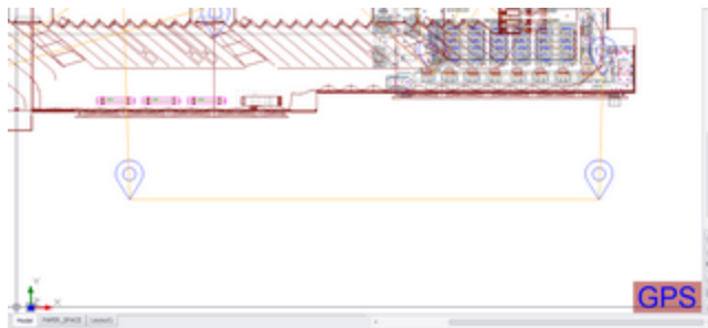
Backbone from panel to panel Via Manhole 1 and Manhole 2
